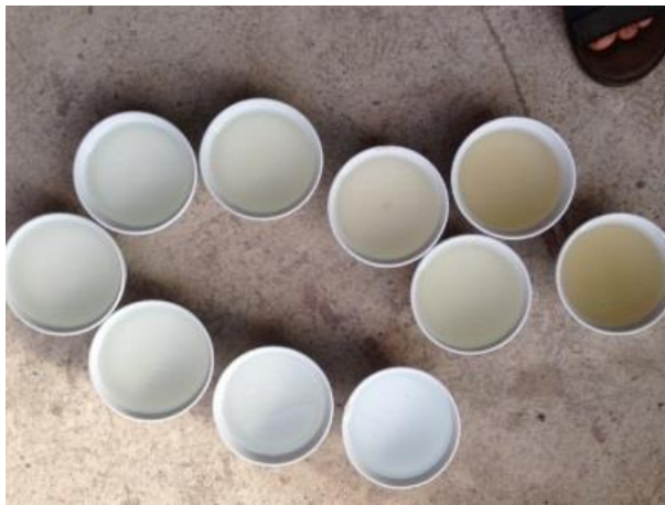
Figure 13: Visual quality evaluation output When the water column H from H = 80 \text{ cm} to H = 0 \text{ cm} .
