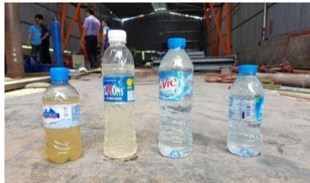
Figure 14: From left to right: input and output with Q = 5 \text{ m}^3/\text{h} ; 4 \text{ m}^3/\text{h} ; 3 \text{ m}^3/\text{h} .
