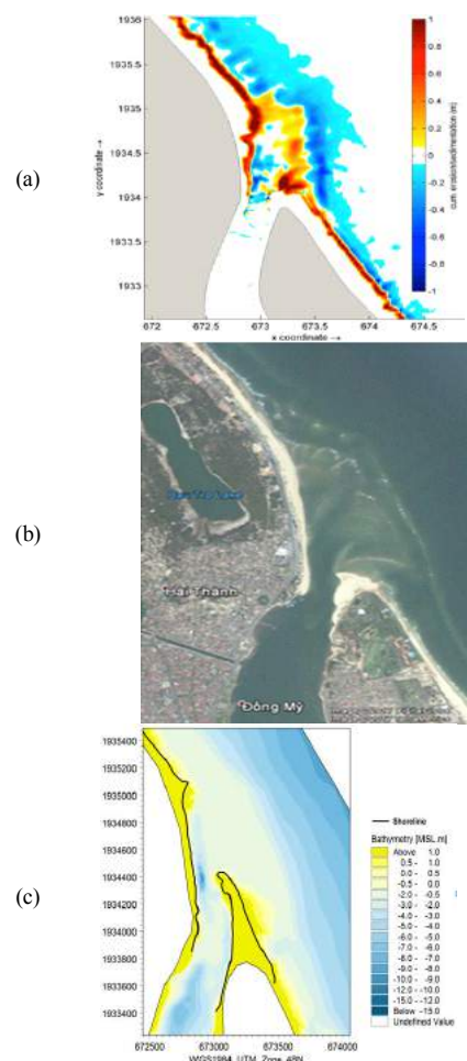
Fig. 9. Erosion/accretion processes are displayed by (a) simulation modeling, (b) Google Earth Image (Screenshot from Google Earth, Map data: Image@2015 Digital Globe, Image@2015 TerraMetrics and Maxar Technologies), and (c) survey data for the flood season in 2015
