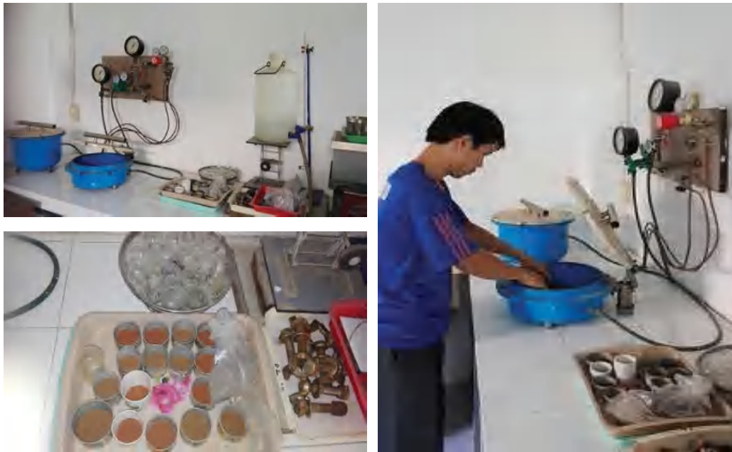
Figure 4: The experiment for determining the water retention curve (pF) for the soil layers
