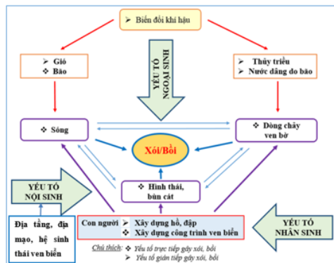
Figure 1.2: Primary causes of coastal erosions and estuary accretions
