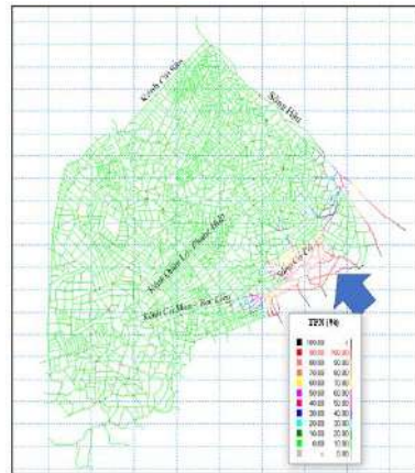
Figure 3.6: Distribution of the composition of sea water from Hau estuary - Hoa Phu channel when there is a salt prevention works (1/2016)
