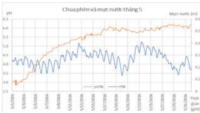
Figure 5: The variations in the pH and water levels over time, at cross-section 96 (branch 30) in May
