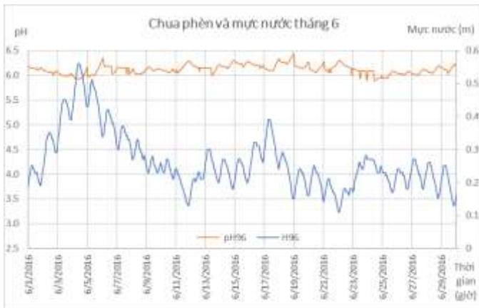
Figure 6: The changes in the pH and water levels over time, at cross-section 96 (branch 30) in June
