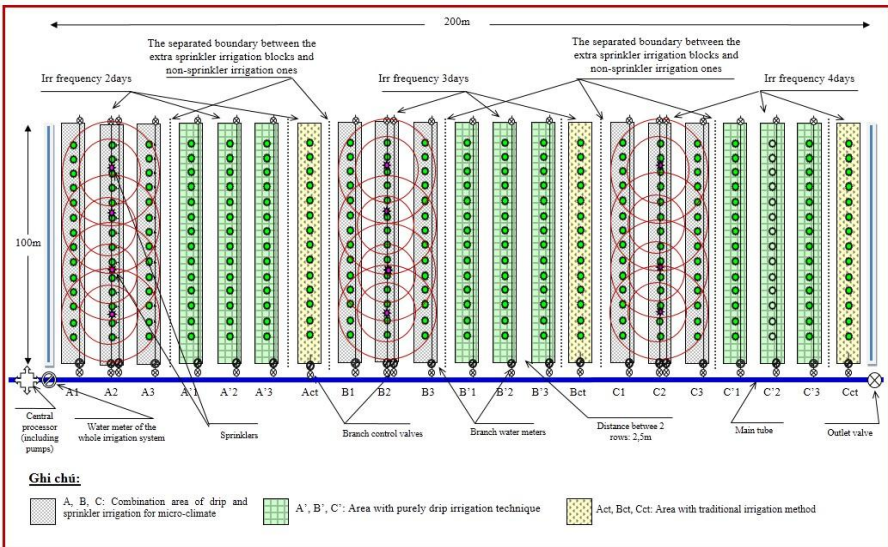
Figure 2.7: The sketch of the experimental model to research on water-saving irrigation schedule for Grape leaves at the scarce region region in the South Central part of Vietnam
