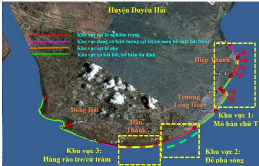
Figure 3. 16: Diagram of orientation of coastal protection structures
